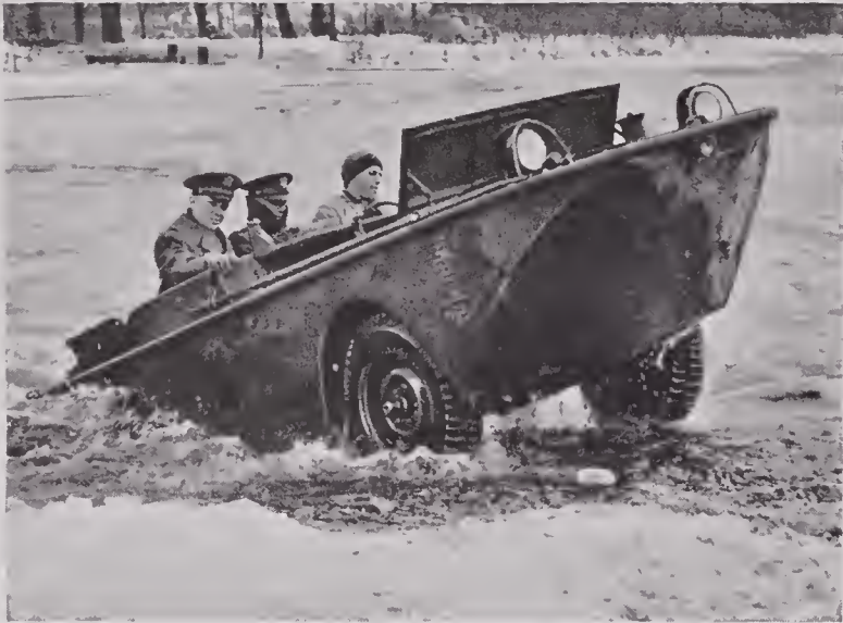
FIGURE 34. Climbing steep river bank, rear deck of amphibious jeep is partly submerged. Most entries down such banks similarly immerse foredeck.
